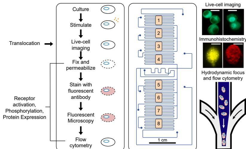
**Figure 2. Microfluidic platform for single-cell imaging and protein profiling.** Microfluidics devices are capable of integrating multiple profiling methods for single-cell characterization, including live-cell imaging, immunohistochemistry, and more detailed characterization following flow-cytometry. Figure courtesy of Anup Singh.
